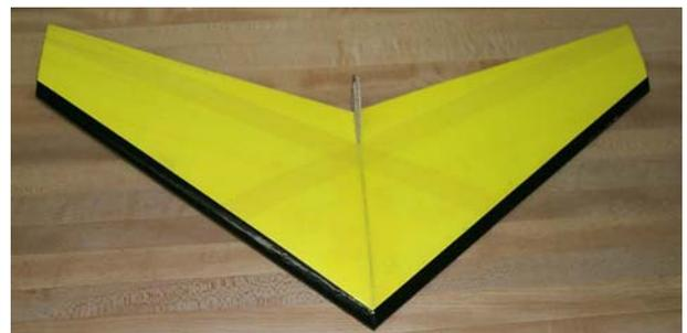
5. Find the elevons in your kit. The elevons are precut, but you have to sand in the bevel on the bottom of the elevon. Also sand an angle at the front of the elevon for clearance.
