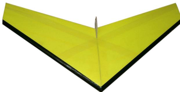
4. Now use a strip of the bottom covering and overlap the top covering at the leading edge.
