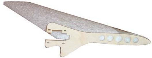
3. Mark the areas where you will recess your radio gear. You can put the gear where ever you like, but here is the recommended location. The servos are placed on top of the wing 2 ½ inches behind the nose and 1 ½ inches to the left and right of the center ply mount. The servo wires are put through the wing and into the ESC hole. The receiver and ESC location is on the bottom of the wing. Also mark where you will route the wires .
