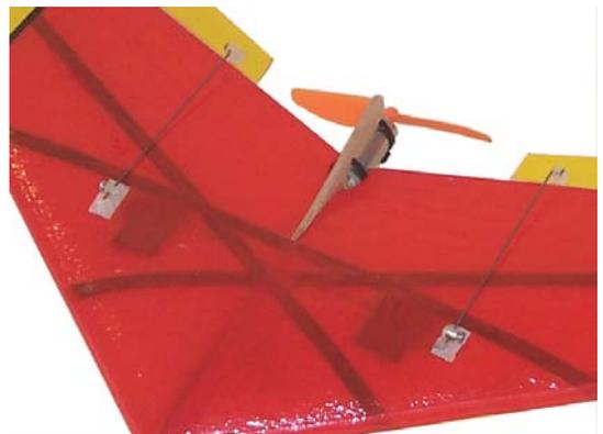
slide the pushrods through the EZ-Connect and tighten the screw making sure that the elevon has a very slight reflex (up angle) to the wing. If you are not using the EZ-
